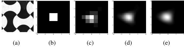
Figure 11. Sub-Pixel PSFs. (a) Cropped section of a sharp image of our grid, (b) PSF (green channel only) at the Bayer resolution (1x), (b) 2x, (c), 8x, and (d) 16x sub-pixel sampling. The sub-pixel PSFs show blur resulting from a combination of diffraction, lens imperfections, and sensor anti-aliasing and sampling.
