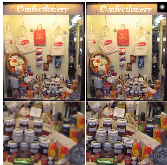
Figure 7. Defocus and Slight Motion-Blur. (top left) The original blurred image and (top right) the deconvolved output with the recovered kernel displayed in the top right of the image (the kernel has been enlarged by 10x for display). (bottom row) Zoomed-in versions of the original and deconvolved image, respectively.
