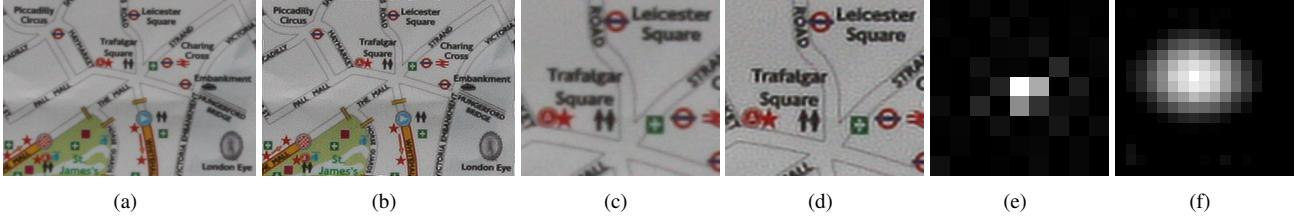
Figure 5. Defocus and Slight Motion-Blur. (a) The original blurred image and (b) the deconvolved output using our recovered PSF. (c–d) Zoomed-in versions of the original and deconvolved image respectively. (e) The kernel recovered using the method of Fergus *et al.* [3] and (f) our recovered kernel.
